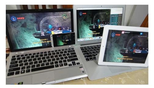
Figure 2: A demonstration of GamingAnywhere system. There are four devices in the photo. One game server (the left-hand side laptop) and three game clients (a MacBook, an Android phone, and an iPad 2). † LEGO Batman software is copyrighted by Traveller's Tales Games Publishing Ltd.
